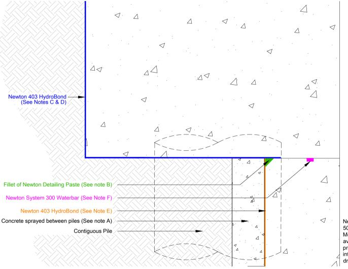
Newton System 500 Cavity Drain Membranes are available to provide Type C internal cavity drainage system
