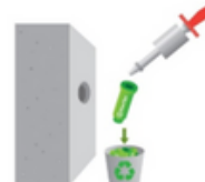
#4 Deposit RivePipe in the bucket for later reuse.
